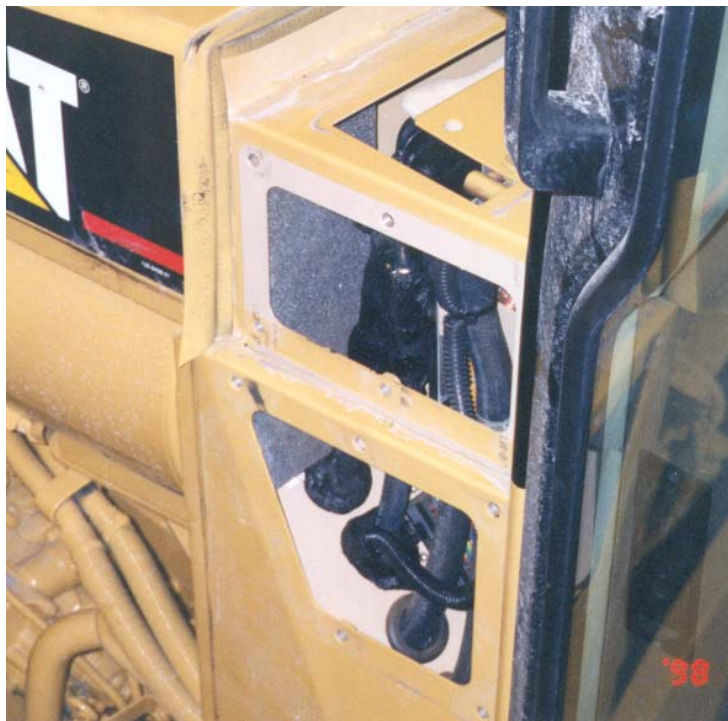
Evaporator assembly showing hoses.
