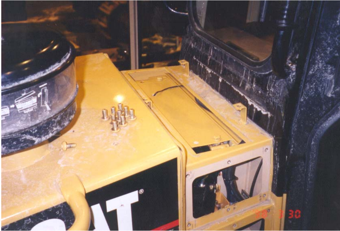
Evaporator cover in place with thermostat.
