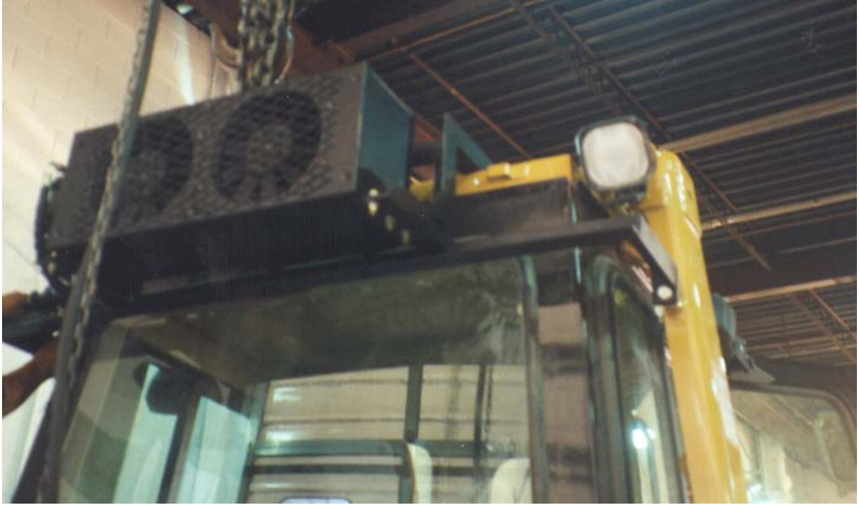
Right side of condenser assembly.(D5M SHOWN)
